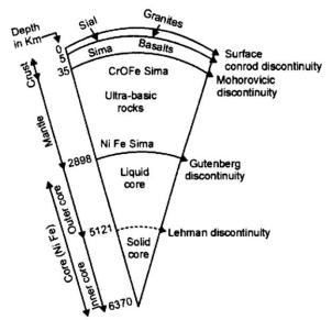
collectively known as the lithosphere, and it is of the lithosphere that the tectonic plates are comprised. Beneath the lithosphere is the asthenosphere, a relatively low-viscosity layer on which the lithosphere rides. Important changes in crystal structure within the mantle occur at 410 and 660 kilometres below the surface, spanning a transition zone that separates the upper and lower mantle. Beneath the mantle, an extremely low viscosity liquid outer core lies above a solid inner core.
